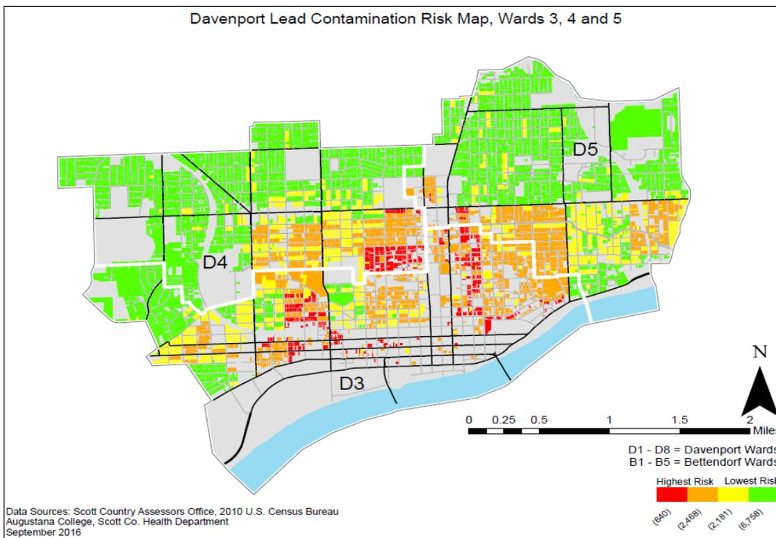
**Figure 3: Example of the detailed scale acquired by mapping at the parcel level. Shown are Davenport city wards 3, 4, & 5.**
