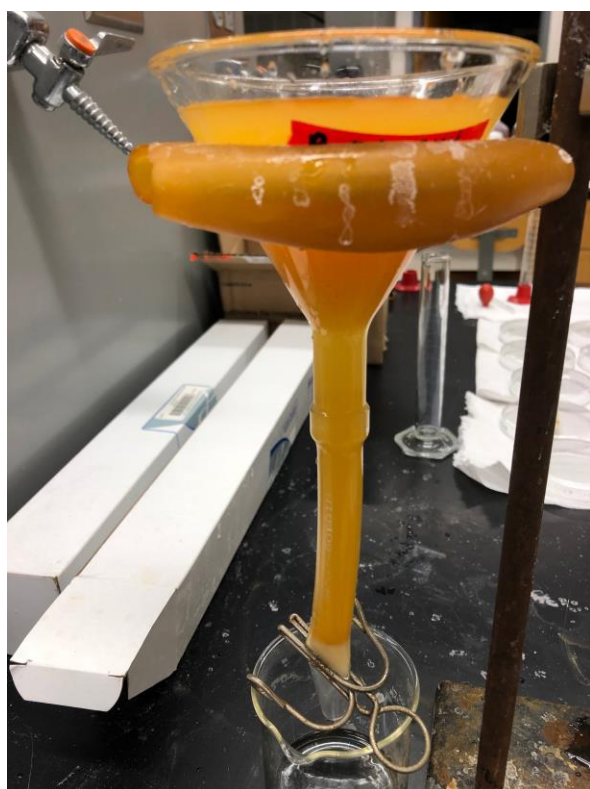
Figure 6: Image A on the left depicts a sample that has undergone digestion and has been mixed with NaCl to facilitate density separation of particles. The image B on the left is the same sample after 24 hours. This time allowed the heavier sediment and particle
