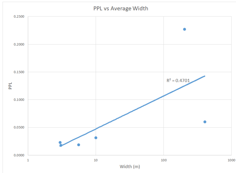
Figure 12: Correlation graph showing a positive relationship between average stream width and plastic particles/liter concentrations
