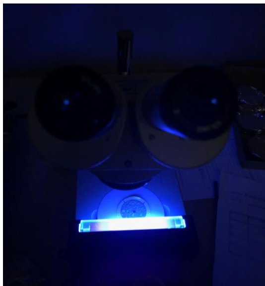
Figure 7: Dissecting microscope, filtered sample, and UV light used to identify plastic particles.
