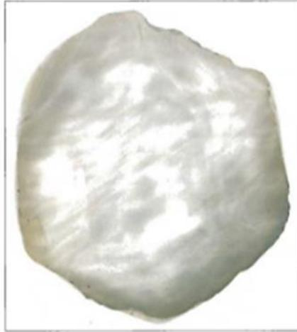
Figure 8. Hercynite precipitation in Fe-rich sapphires from Rock Creek, Montana due to heat treatment in over reducing conditions. Prior heat treatment, the wafer was colorless and transparent and after heat treatment, it turned translucent gray (Emmett et al., 1993).
