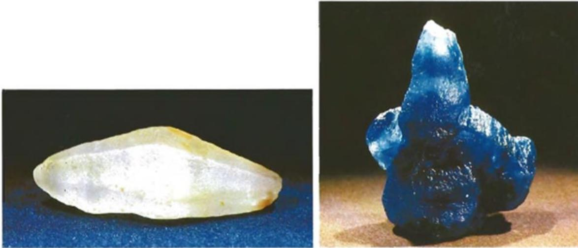
Figure 6. Left, milky white (geuda) corundum from Sri Lanka heat-treated under reducing conditions to deepen the blue color and improve clarity. Right, is the result of heat treatment under reducing conditions. From (Nassau, 1981).
