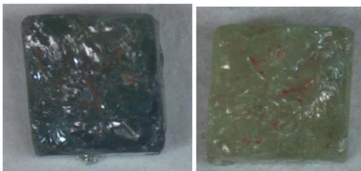
Figure 20. C2-1 sapphire pre-heat-treatment (left) and post-heat-treatment (right). The dark brown filled inclusions changed to dark red (transition from goethite to hematite)
