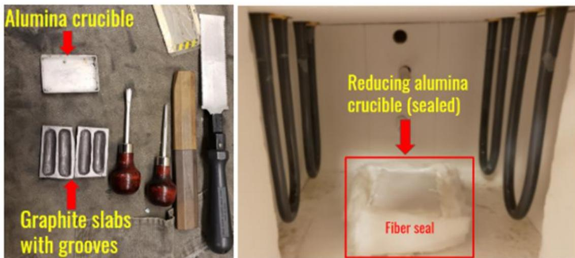
Figure 12. Graphite slabs with boat-shaped grooves and alumina crucible on top (left). Two alumina crucibles with two graphite slabs facing each other while housing corundum stones. Sealed off with alumina fiber. Also the inside of the furnace (right).
