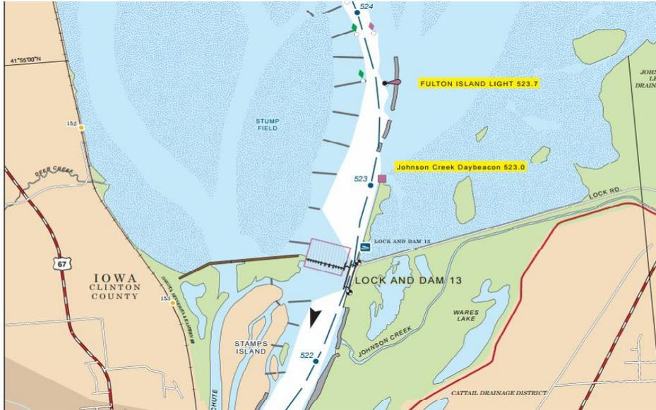
**Figure 2. A map of the river near Lock and Dam 13 illustrates the impact of dam construction on islands (USACE, 2012). Upstream of the dam, the areas shown as “stump fields” mark the locations of former islands that have been drowned or eroded following the dam construction. By contrast, islands persist in the river reaches immediately below each dam (see Stamp’s Island for example).**
